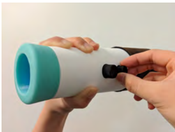
Figure 4: In addition to the rotary wheel, two knobs are designed aside for the interactive setting.
