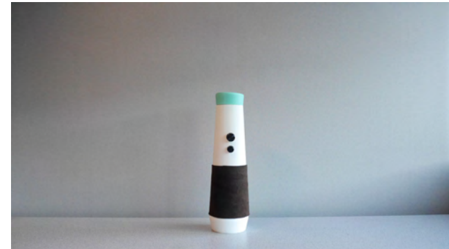
Figure 1: Chronoscope is a telescope-like Research through Design [5] artifact that enables people to view their digital photo collection on a display inside and to interact with it by rotational controls.
