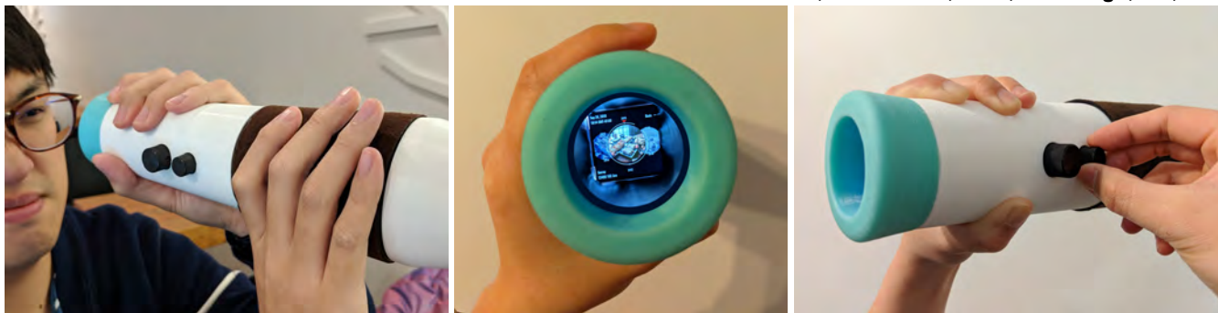
Figure 2: Left: Using his right hand the user manipulates a fully rotational black silicon surface (rotating clockwise moves ‘forward’ in time and rotating counter-clockwise goes deeper into the past). Middle: Peering into the turquoise eye piece through a magnification lens, the user views photos from his past. Right: The user manipulates a black metal knob that ‘tunes’ the granularity of photos that moved through in each rotation; the untouched knob toggles between timeframe modes.
