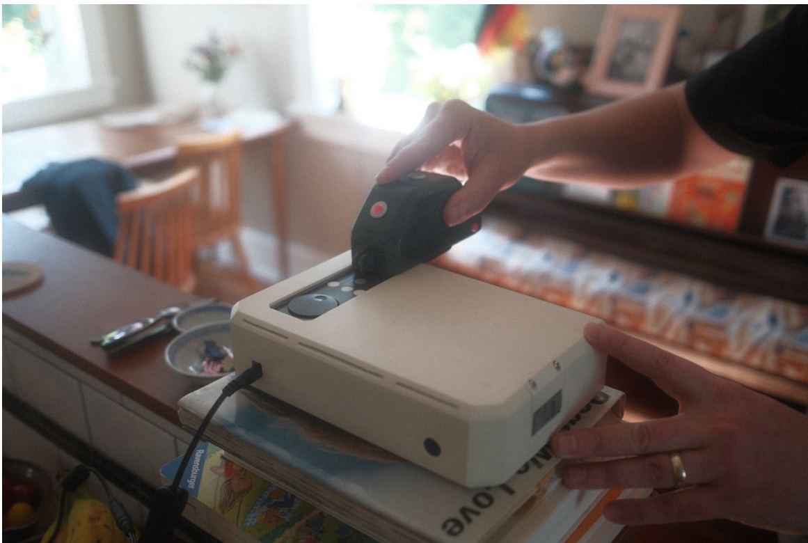
Figure 2: The Capra Collector sliding into the Capra Explorer. This action triggers data transfer of recently collected hikes on the Collector into the archive of all hikes stored and viewed on the Explorer.
