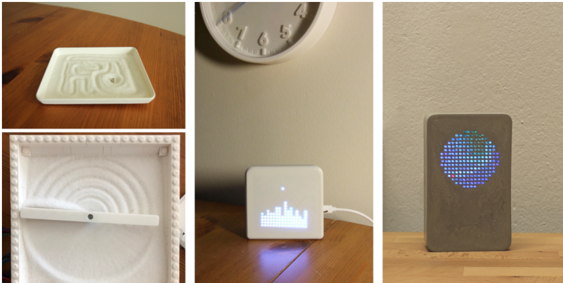
Figure 4.18 The 3 major forms for Memory Tracer. Sand tracer form (left) would trace a pattern representative of a location. Hourglass form (center) showed time flowing through the device as it surfaced a moment. Final form (right) slowly revealed a trace of a map showing both location and time flowing through the device.
