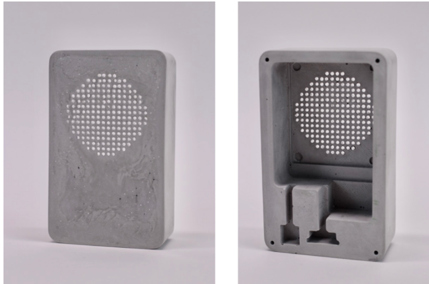
Figure 4.19 Final form, casted from Rockite with embedded fiber optic cables to allow light to pass through the concrete
