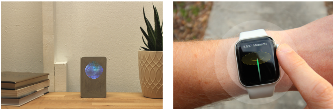
Figure 1.1 Memory Tracer (left) is a device that occasionally surfaces location moments from the past bound to today's date. Memory Compass (right) is a smartwatch application that uses a 'casting' interaction metaphor that enables a user to retrieve and explore location moments from their past, across space and time
