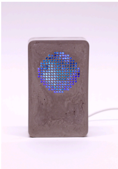
Figure 4.13 The design process ultimately led to this final form, guided by the following goals: 1) does not look like merely an enclosure for a screen, 2) invites peering into, 3) feels durable and weighty
