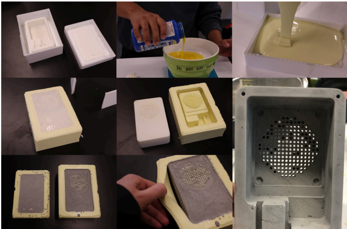
Figure 4.11 The various stages of mold making and casting. The final form was cast using Rockite cement.
