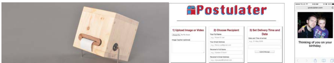
Figure 7: Reflexive Printer prints a halftone photo from its user's smartphone on thermal paper, and deletes it; Postulator is an online application that allows users to send multimedia messages, including images or videos, to a future date and time. Images retrieved from Tsai et al.'s paper in 2014 [223] and Hawkins et al.'s paper in 2015 [87]
