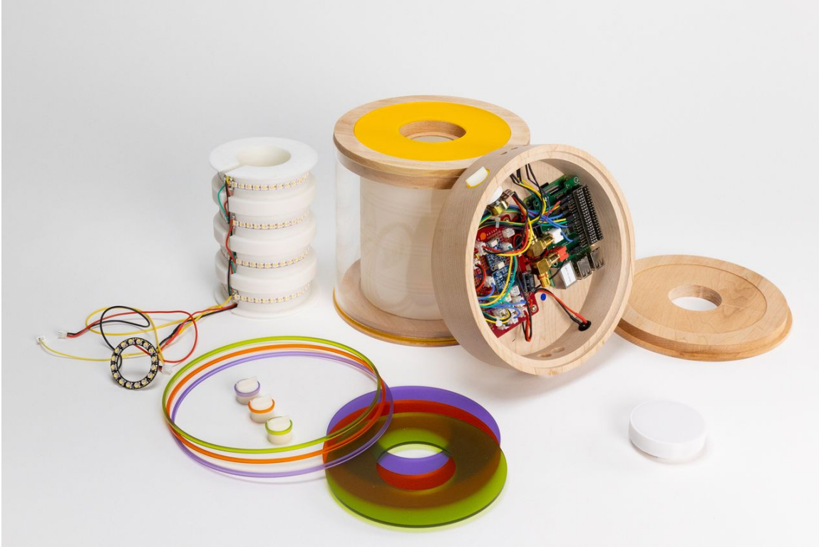
Figure 3.30 The main components of Queue Player from left to light: RGBW ring light, core for RGBW LED strips, resin printed knobs, frosted acrylic tops, a transparent acrylic Tube, a wooden base and top made from maple, final electronic and hardware implementation, a 3D printed disc to diffuse the RGBW ring light
