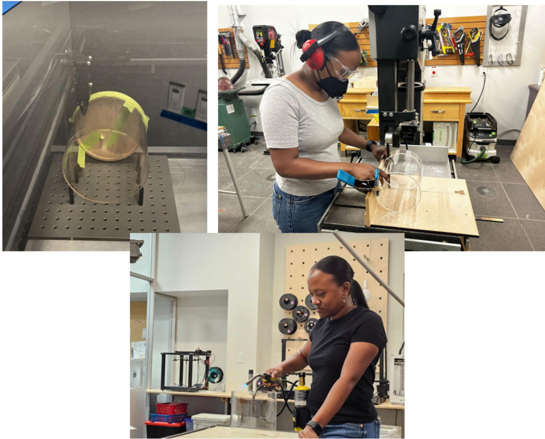
Figure 3.25 In the meantime, I moved on to cutting the acrylic tubes for each Queue Player's outer shell. At first, I tried to use our laser cutter to achieve smooth and uniform edges. However, it was difficult to do this without a rotary attachment. I ultimately used the bandsaw to cut the tubes, but was left with very rough edges. Using a propane torch to flame polish the edges gave me a much cleaner finish.
