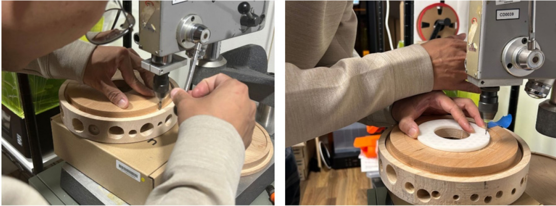
Figure 3.24 Henry Lin and I also drilled holes to connect all of the Queue Player components together. This process was a major encounter and pause , as it took us a while to come up with the optimal solution for connecting everything. Drilling these holes also required a precision which had never been used for anything like this before.
