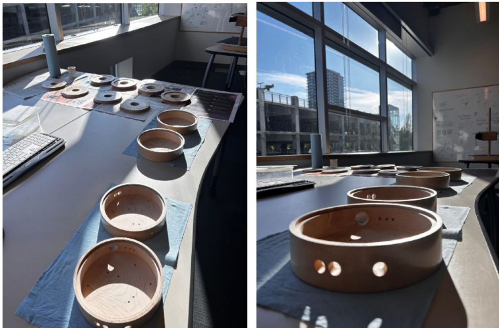
Figure 3.23 I polished the maple using a glossy hardwax oil. Waiting for them to dry between coats was another pause . We were unable to move ahead with integrating all of the components until these were completely dry.
