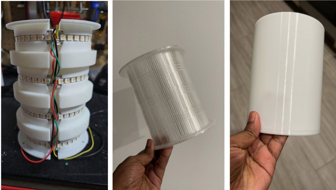
Figure 3.18 I designed a cylindrical core for to embed lights for the queue (see left). I also began to explore different forms and material options for a light diffuser. Early attempts used 3D printed PLA (see middle and right). Translucent filament resulted in undesired light refraction, while the white was much closer to want I pictured. However, I still felt that the ridges from the 3D printed layers were too distracting.
