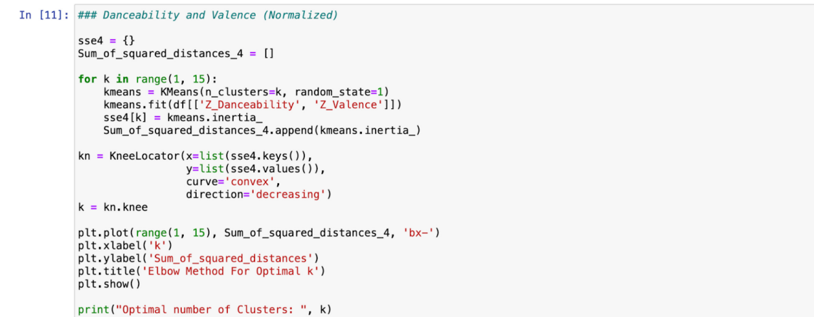
Figure 3.11 Using k-means to calculate the optimal number of song clusters
