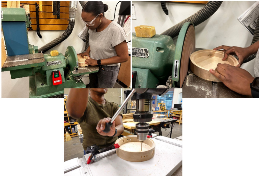
Figure 3.21 I then sanded all of the wooden components and drilled holes to mount the electronic hardware, knob, indicator light LEDs, and plugins for power and RCA.
