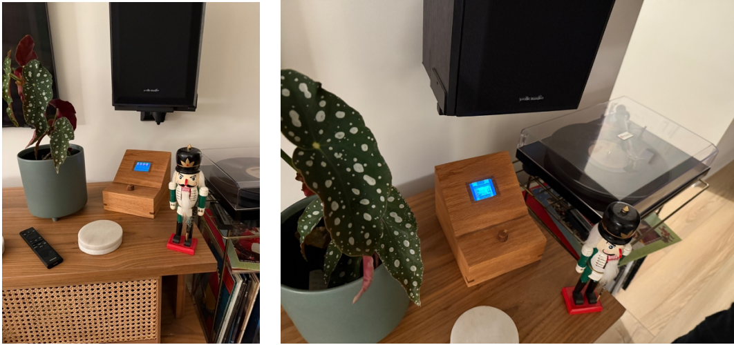
Figure 3: The ‘vinyl scrobber’ handcrafted by P1 composed of mahogany wood, a Raspberry Pi and small display paired with a mobile application for logging vinyl listening histories manually.
